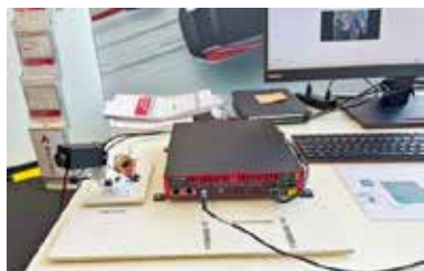
Image 1: Demonstration setup: A VN5650 with integrated KD's optical KD7251 PHYs is shown with its optical connectors. In the setup, the PHYs are looped to transfer gigabit camera data live.
