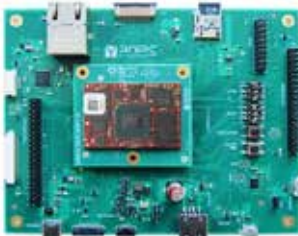
Image 3: MSRZG3EEVK evaluation board by ARIES Embedded with Renesas RZ/G3E MPU for rapid prototyping and quick project entry
