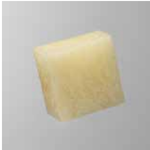
Image 1: HyTemp® ACM from ZEON is a specialty oil-resistance rubber for high temperature application
