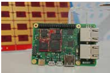
Image 1: ARIES Embedded presents FIVEberry baseboard for broad and easy access to RISC-V technology
