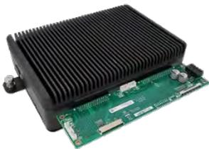
Image 2: BoxPC Pro NPA-2009 from Distec with V-by-One and eDP interface and Docking Connector
