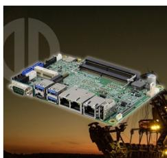
Image 1: Robust IB836 single board computer from iBASE with Intel x6000 available in Distec's industrial portfolio
